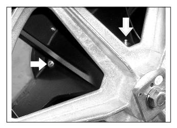
■ After about 1000 operating hours, lubricate the drum journal bearings with the lubricating nipple using Arcanol L 100 grease.
